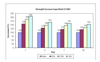
In cases when concrete is applied at high ambient temperatures or prolonged transportation of concrete is required, recommended dosage are above 0,8% and class of consistency should be S4 or S5; At normal temperatures (up to 25<sub>°</sub>C), concrete produced with Superfluid 21 EKO, can be transported and applied with pump in period up to 60 minutes.
